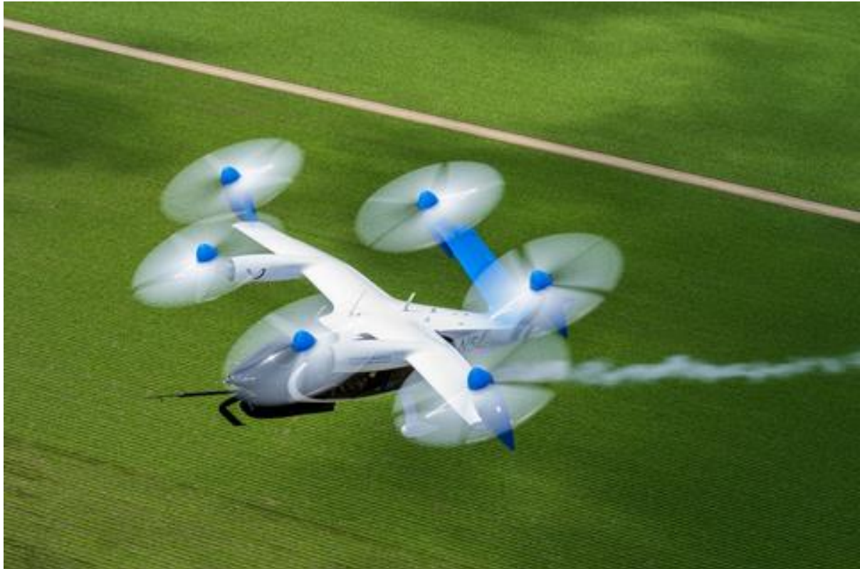
Figure 23 - Joby 4 passenger eVTOL demonstrator
