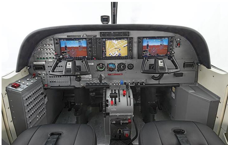
Figure 10 - Cessna Caravan new aircraft flightdeck
